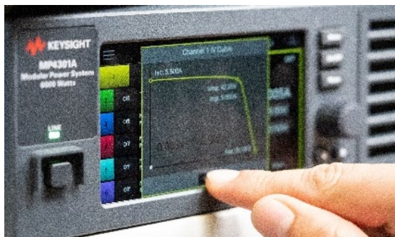
Figure 4. Intuitive touch display, setting SAS curve
