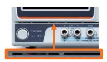
There are air inlet ducks in front of the panel to efficiently dissipate heat. Temperature controlled fan can effectively reduce fan noise.
