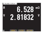
Simple Mode (R+V measurement parameters)
